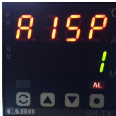
You can now or at any time during the firing process press the
